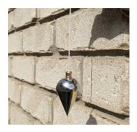
A **plumb line** is a tool that people still use today. The top is attached to the scaffolding at the top of the building and the bottom aims at the center of the earth by gravity, making it always straight and true.
